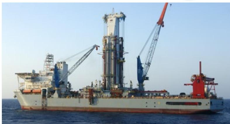
The vessel Globetrotter II is a drilling Ship built in 2012 and currently sailing under the flag of Liberia. It's 620 ft. long, with a drilling depth of 40,000 ft.
